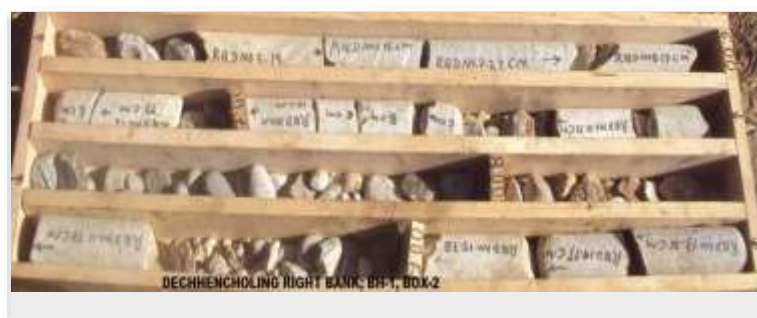
Figure 7: Samples of the cores from borehole at right bank
