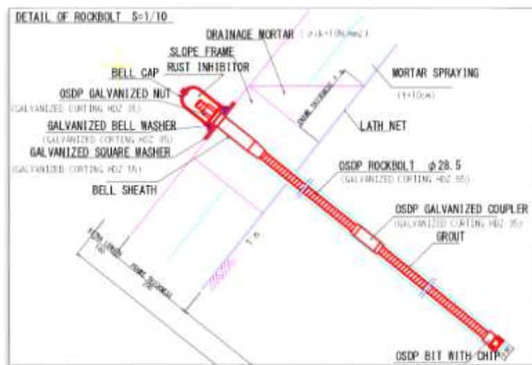
Figure 4. Detail of Soil Nailing Component
