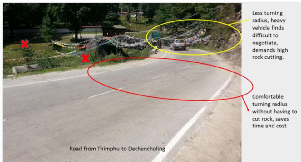
Figure 3: Comparison of turning radius of old bridge and propose bridge location
