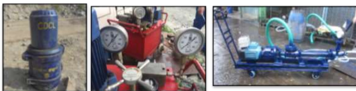
Figure 17: Post tensioning equipment (stressing jack, pressure pump, grouting pump).
